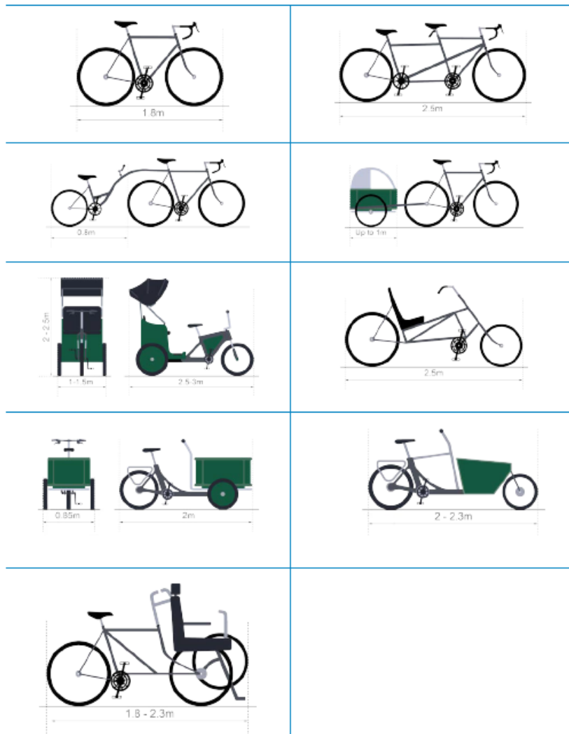
Figure 2: Typical dimensions of cycles (Source: Cycle Infrastructure Design, Local Transport Note 1/20, July 2020, Figure 5.2)
